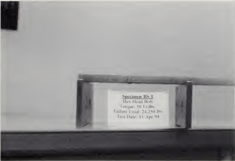
Specimen BS-1, Hex Head Bolt, 50 ft-lbs torque. Edge view, GRP panel, showing moderate brooming.
